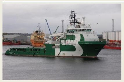
The Ulstein A102 **Bourbon Dolphin** entered service in late 2006 and capsized with the loss of eight lives while anchorhandling at the **Transocean Rather** in April 2007. This then might be the only claim to fame for the vessel type, of which no more have been constructed. It appears that the intent of the design was to produce a high specification vessel in a smaller hull than the Ulstein A101, and here I might have to declare a
