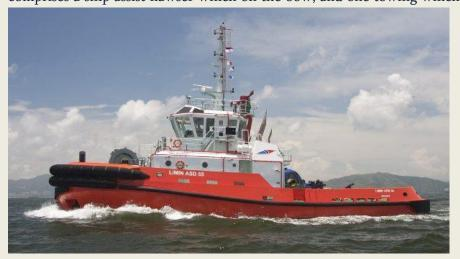
knuckle boom deck crane is installed on aft deck for handling of service parts and small cargo. Main propulsion for each tug comprises a pair of CAT 3516C diesel engines, each rated at 2682 BHP at 1600 rpm, and each driving a Schottel, SPR 1515 fixed pitch Z-drive unit, in ASD configuration. The electrical plant comprises
