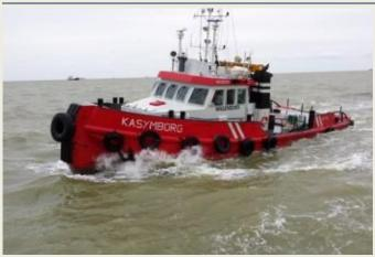
generates 23.5 tonnes of bollard pull. Equipped with a crane. **Kasymborg** is often deployed as a service vessel, such as recently for dredging company Jan de Nul. Their Multicat **DN 34** was towed successfully from Turkmanbashi to Aktau by **Kasymborg**. (*Press Release*)
