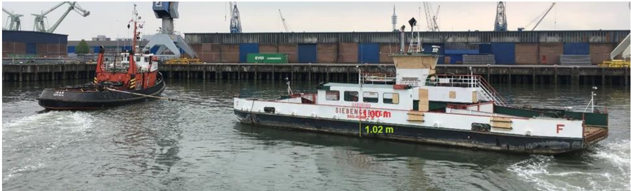
Photograph 11: Ferry's freeboard: FB = 1.02\text{ m}
