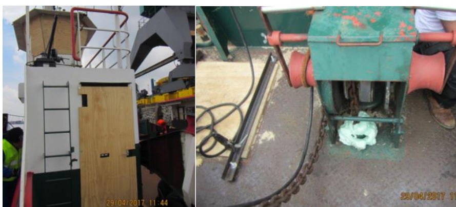
Photograph 8: Door to the superstructure – starboard. Sealing of the chain pipe. Compartment No 2
