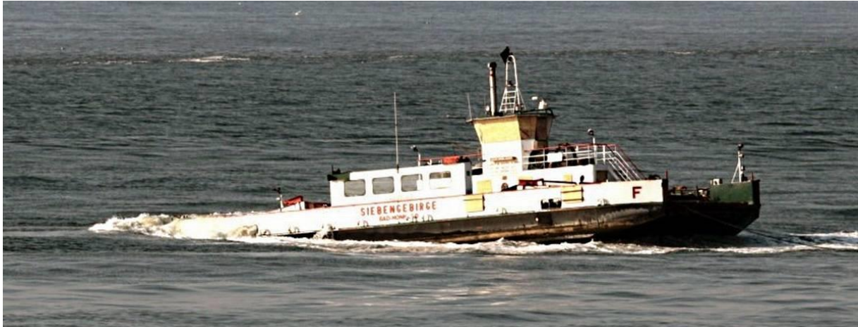
Photograph 13: The „Siebengebirge” ferry with the bow under water. The photograph presents the stern – portside of the ferry. One can see the outflow of water from the deck ( http://www.general-anzeiger-bonn.de )
