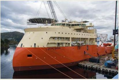
On Tuesday night, yard number 302, Island Ventue, an offshore construction vessel for Island Offshore/Edison Chouest Offshore, was launched from the dock hall at Ulstein Verft. Currently, the heli deck is being mounted. Measuring close to 160 m in length, and with at beam of 30 m, she is the largest offshore vessel so far from Ulstein Verft. The vessel is jointly owned by Norwaybased Island Offshore and US-
