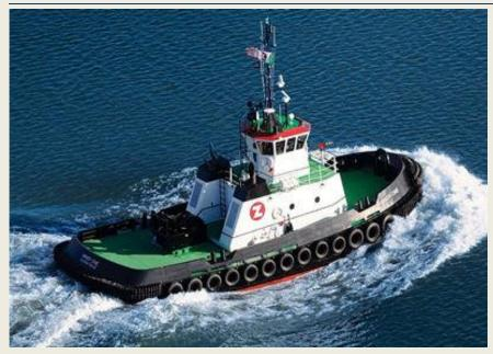
Great Lakes Shipyard, a division of The Great Lakes Towing Company, Cleveland, Ohio, celebrated the signing of a construction contract to build another of its HandySize Class, 3,400 HP twin-screw tugboat for harbor towing operations Quetzal; in Puerto а growing principal commercial cargo, container, and cruise port located on the Pacific coast of Guatemala in Central
