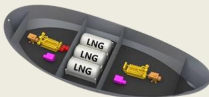
*Dual-Fuel Diesel-Direct drive*
