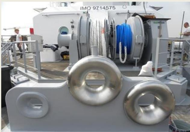
On the foredeck we see the anchor winch with a 5 tons capacity capstan.
