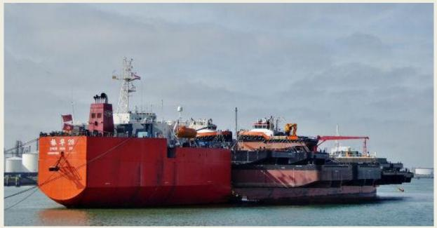
cargo vessel *Zhen Hua 28*. Several pontoons were seen on deck with on top two Damen Shoalbusters and three small tugs. *(Photo: Jan Oosterboer.)*
