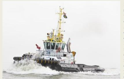
LEADING towage and salvage specialist Multraship has welcomed Multratug 28, an energy-efficient hybrid Damen ASD 2810-type tug with stateof-the-art FiFi 1 firefighting capabilities, into its fleet. Damen's ASD 2810 Hybrid is a new design and this is the second of its class to be built. It features diesel-direct, dieselelectric and battery-powered propulsion systems. This hybrid configuration will enable
