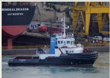
The tug has length of 32.50 mtrs a beam of 10.80 mtrs and a depth of 5.60 mtrs. The two GE Marine type 7FDM12 develops a total output of 4,360 kW at 1,000 rpm. She has a free sailing speed of 14 knots and a bollard pull of 80 tons ahead and 75 tons astern. She is classed Registro Italiano Navale. *(Photo: Capt. Lawrence Dalli - www.maltashipphotos.com)*
