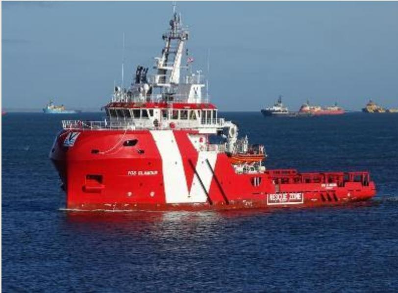
while making for a handsome distinctive look. The mechanical-driven vessel also boasts of lesser vibrations and noise levels, as confirmed through rigorous testing and crew feedback. Other features include anti-rolling tanks for increased performance and crew comfort in extreme weather conditions, as well as a retractable bow thruster for easy manoeuvrability and reduced fuel consumption during daunting rescue missions. Spacious
