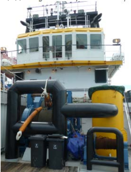
diesel engines for a bollard pull of 42 tons, further more a Double drum towing winch 50/75 tons is installed and the tug can carry 290.000 litres of
