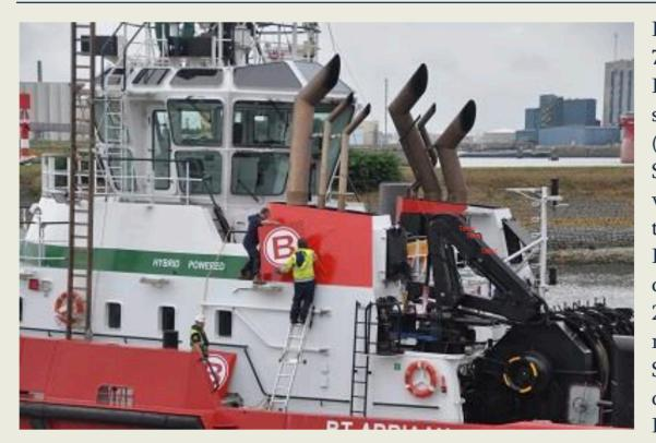
In the afternoon September 7th, was seen the 2010 built Dutch registered with call sign PCWG tug RT Adriaan (Imo 9489936) moored in the Scheurhaven, where the "K" was replaced by the "B" in the funnels. The Rotor Hybrid tug has a length o.a. of 32.00 mtrs a length bp of 29,07 mtrs a beam of 12.00 mtrs and a depth 6,45 mtrs. She performed a bollard pull of 84 tons. She is classed Lloyds Register of Shipping.
